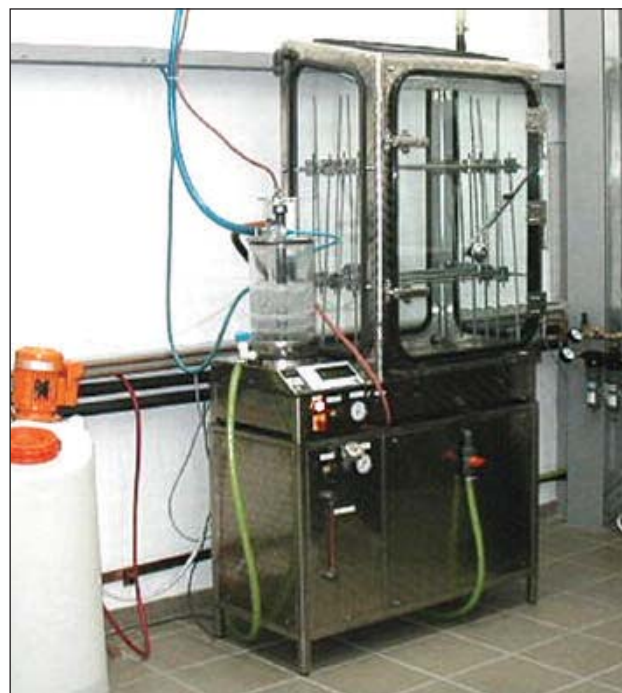
Environmental ageing chamber for ammonia atmosphere ageing
