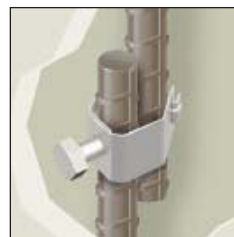
Figure 14: Typical methods of bonding to steel reinforcement within concrete
