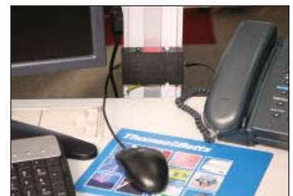
An ESP TN/RJ11-4/6 protecting an external fax line. Note the short earth connection made to the local ring main
